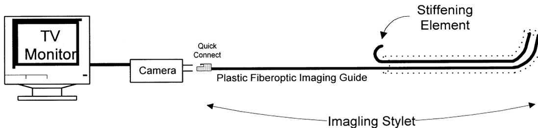
Fig. 1. This diagram shows the components of the plastic fiberoptic imaging system. The stiffening element is inserted into an endotracheal tube and is formed to the desired shape. During laryngoscopy, the airway structures are viewed on the TV monitor and the endotracheal tube with imaging stylet is manually steered between the vocal cords and into the trachea.
