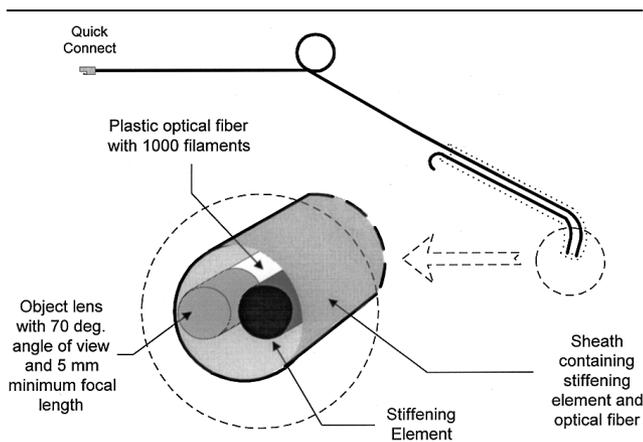
Fig. 2. An illustration of the components and specifications of the imaging set.
