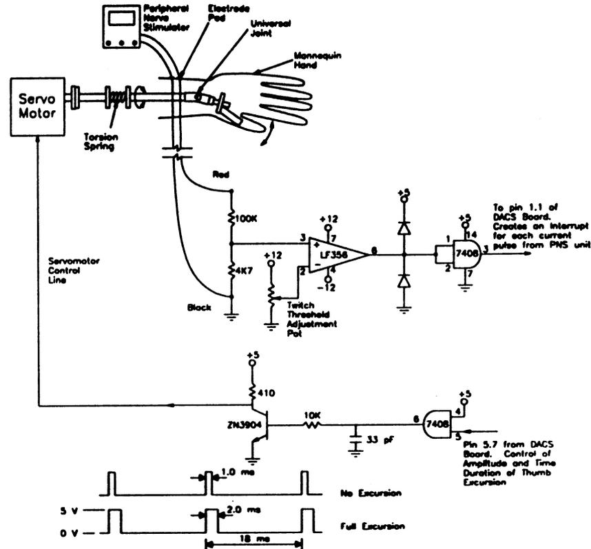
Fig. 2. The detailed schematic of TWITCHER.
