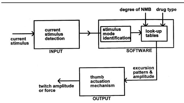
Fig. 1. The high level block diagram of TWITCHER.
