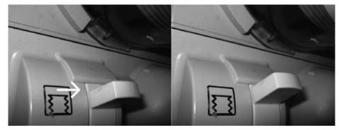
**Figure 1.** View (from above and left) of the absorber housing and the Bag-Ventilator switch short of its mechanical limit (arrow in left picture) and at its mechanical limit (right picture). From the typical perspective of an anesthesia provider, the difference in selector switch position will be less noticeable.
