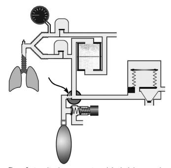
**Figure 2.** A stylized representation of the leak between the manual and mechanical ventilation sub-systems that occurs only when the failed selector switch is in the mechanical position. Based on the Virtual Anesthesia Machine (VAM) simulation http://vam.anest.ufl.edu (with permission from the VAM authors).
