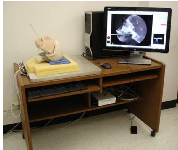
Figure 7: The RFL mixed simulator. It comprises the phantom head, the electromagnetic tracker (the gray metallic plate underneath the phantom head) with electronic controller, and the computer that simulates the fluoroscopy unit.
