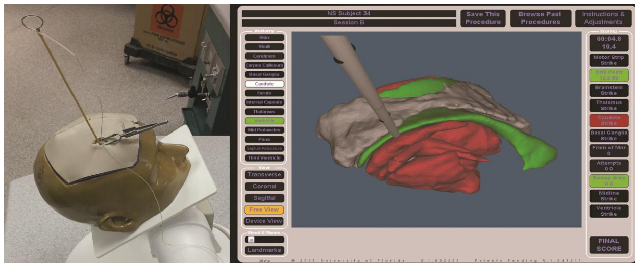
Figure 5. Left: The mixed reality ventriculostomy simulator; a catheter stylet tracked in 3D space is inserted via a hole drilled by the learner through a disposable skull insert and steered to the ventricle. Right: The virtual soft tissues (ventricles, caudate, brainstem and other inner brain components) are displayed collocated to a virtual representation of the physical catheter/stylet. The scalp, skull and outer brain opacity have been set by the instructor to transparent, in this view. The ventricles are colored green in the display.
