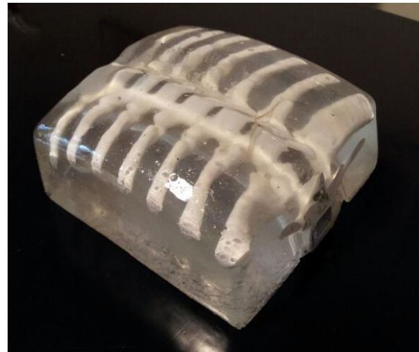
Figure 12. The physical spine segment embedded into ballistic gel.
