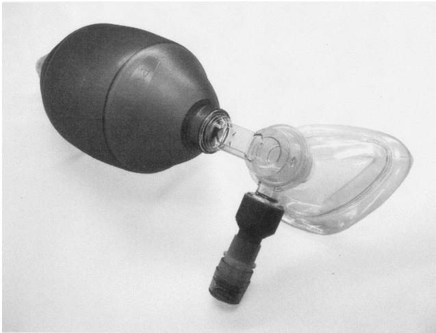
Figure 1. Self-inflating manual resuscitator with reed whistle on exhalation port used for study. The reed whistle is at the bottom of the photograph.
