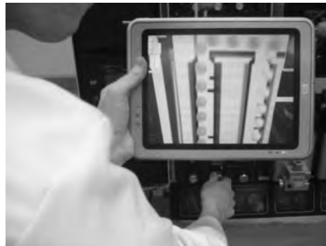
Fig. 9. A user turns the N_2O knob on the real machine and visualizes how this interaction affects the overlaid VAM model.
