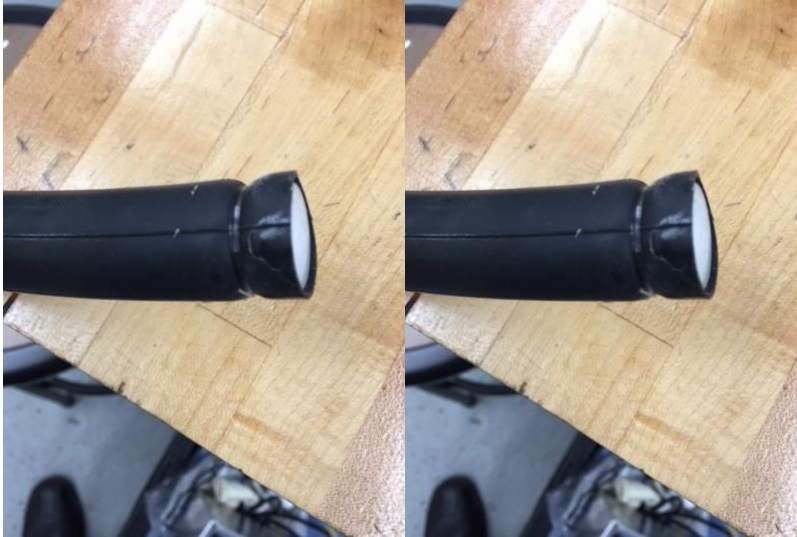
this image shows a nylon wrap that is too tight with a groove that is too deep, and may have caused premature failure
