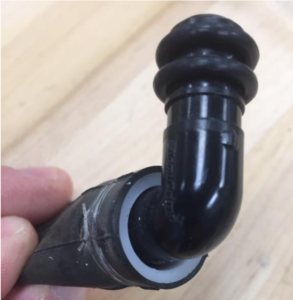
Completed Assembly of Valve that will sit within Sections O T and U of the ventilator assembly
