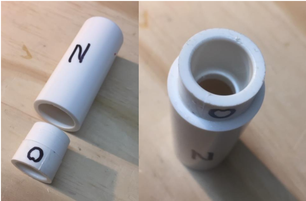
Use silicone adhesive on mating surfaces of part N and O
