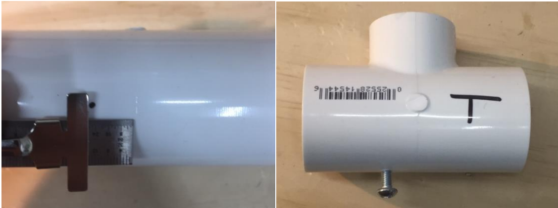
Drill 9/64" diameter hole 14/32" to 1/2" from centerline of T as shown, install #8-32 x 1/2" screw
