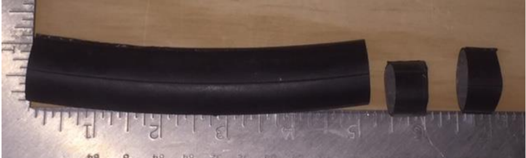
5" and two 1/2" sections of butyl rubber tube
