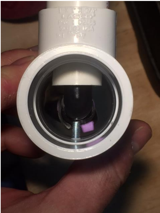
#8-32 x 1/2" screw holds elbow against air pressure during inhalation
