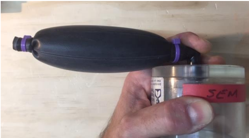
Leak test. Do not overinflate, can be done underwater
