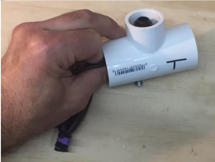
Hold exhalation bulb in place and slide in N and O assembly
