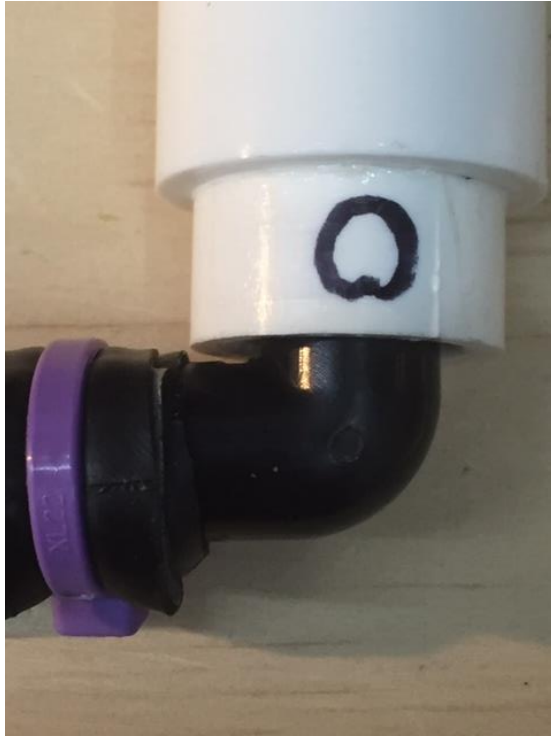
O-rings (inside, not shown) form tight seal between elbow R and O.
