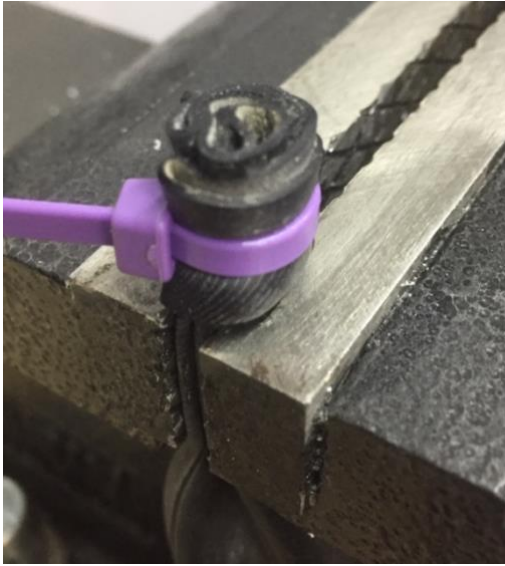
Cable tie over ½" section of tube. Cable tie must have no direct contact with 5" tube.
