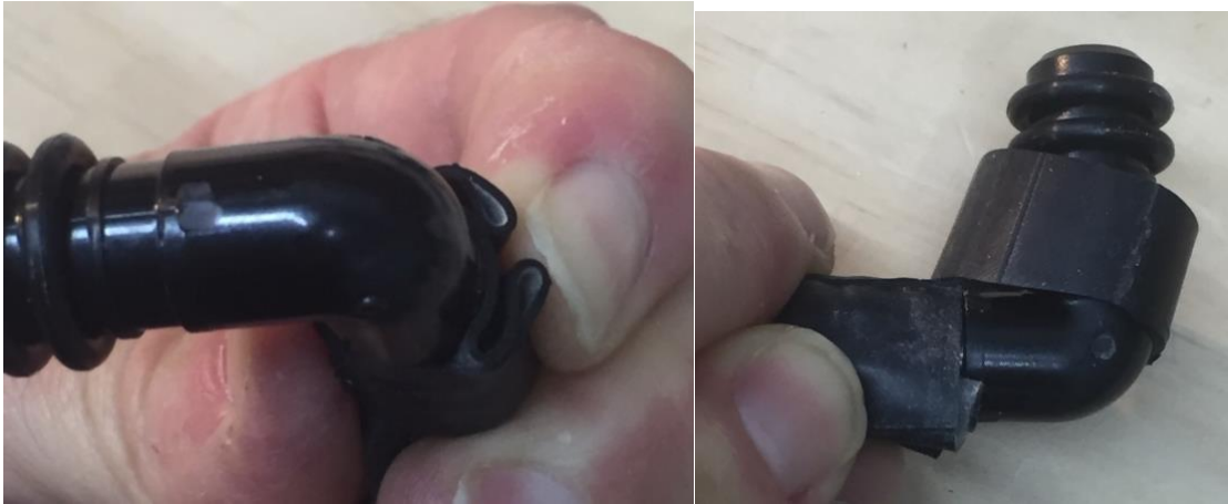
Pinch and wrap 5" section around elbow, have 1/2" section in place.
