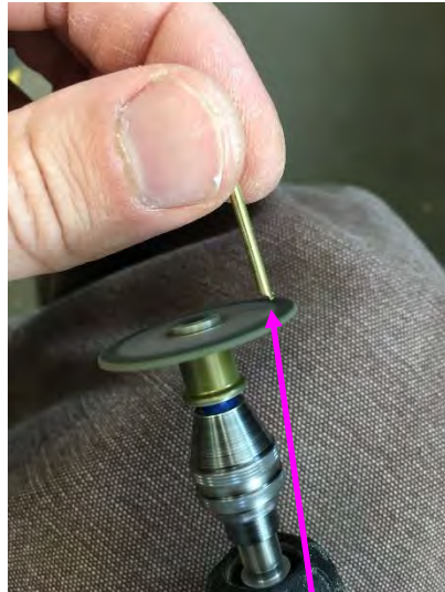
Use cutoff wheel carefully or use sandpaper to flatten and square the end of the tube.
