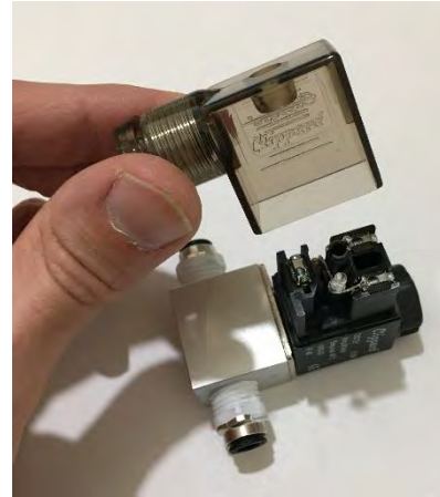
Plastic housing should pull off.. It is possible the black terminal lug section could come off with it.
