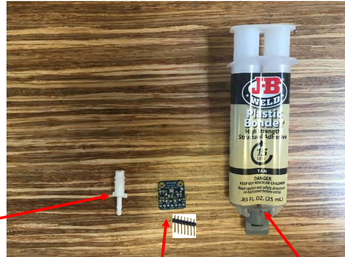
Adafruit BMP280 sensor and 7-pin header
