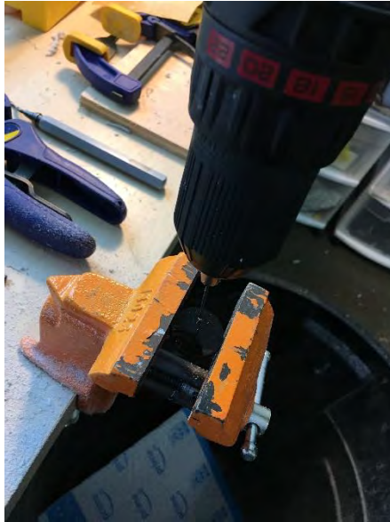
#55 drill bit (0.052 in) (1.3208 mm)
