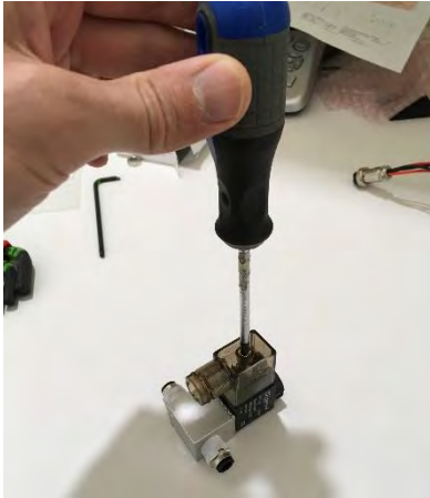
Unscrew the screw in the plastic housing.
