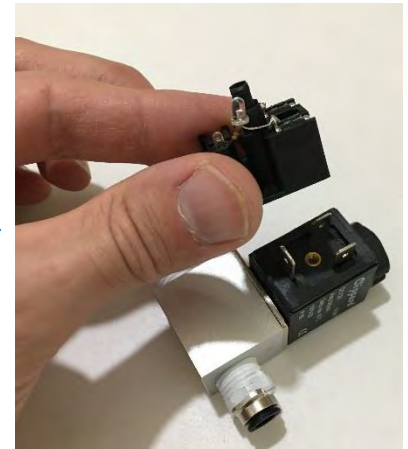
Pull off the black terminal lug section.
