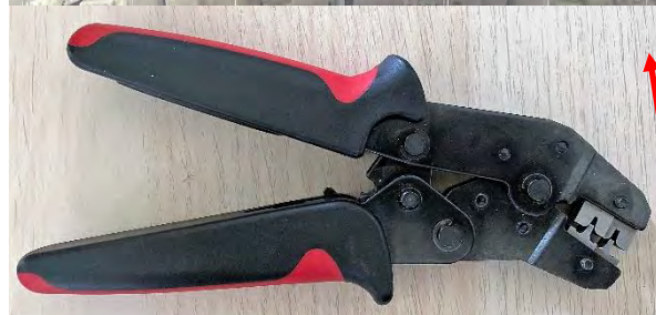
JST-XH Connector Kit with Crimping tool
