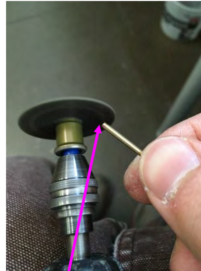
Very lightly bevel the corners of the brass tube.
