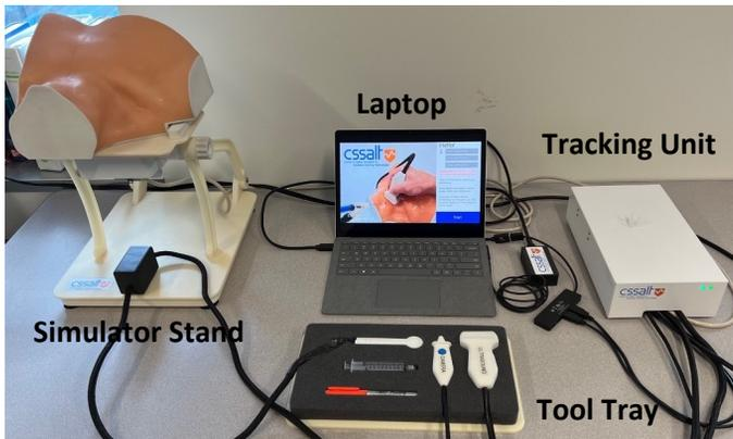
Keep the Simulator Stand away from the Tracking Unit by 4 feet or more; the electromagnetic tracking system is sensitive to metal.
