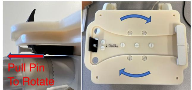
To rotate the top platform, pull the latch pin outwards and then rotate. Friction when rotating is normal, it is easier to use both hands holding opposite side of the platform to rotate. The latch pin is to prevent unwanted movement.
